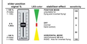
Slider more towards the center reduces the sensor gain and slows down the corrections.
