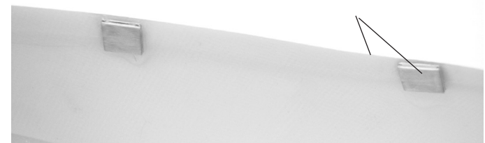
Blocks mounted flush to the canopy edge.
